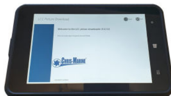
A hand-held tablet, also compatible with the Chris-Marine LDM, is used to collect picture data from the LCC unit. It is also used to take pictures of ring pack and top/land.
