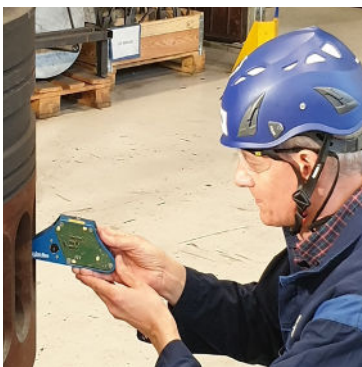
The LCC unit and its base are easily inserted through a scavenge air port.
