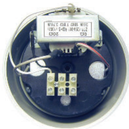
Electrical connector inside sound emitter housing
